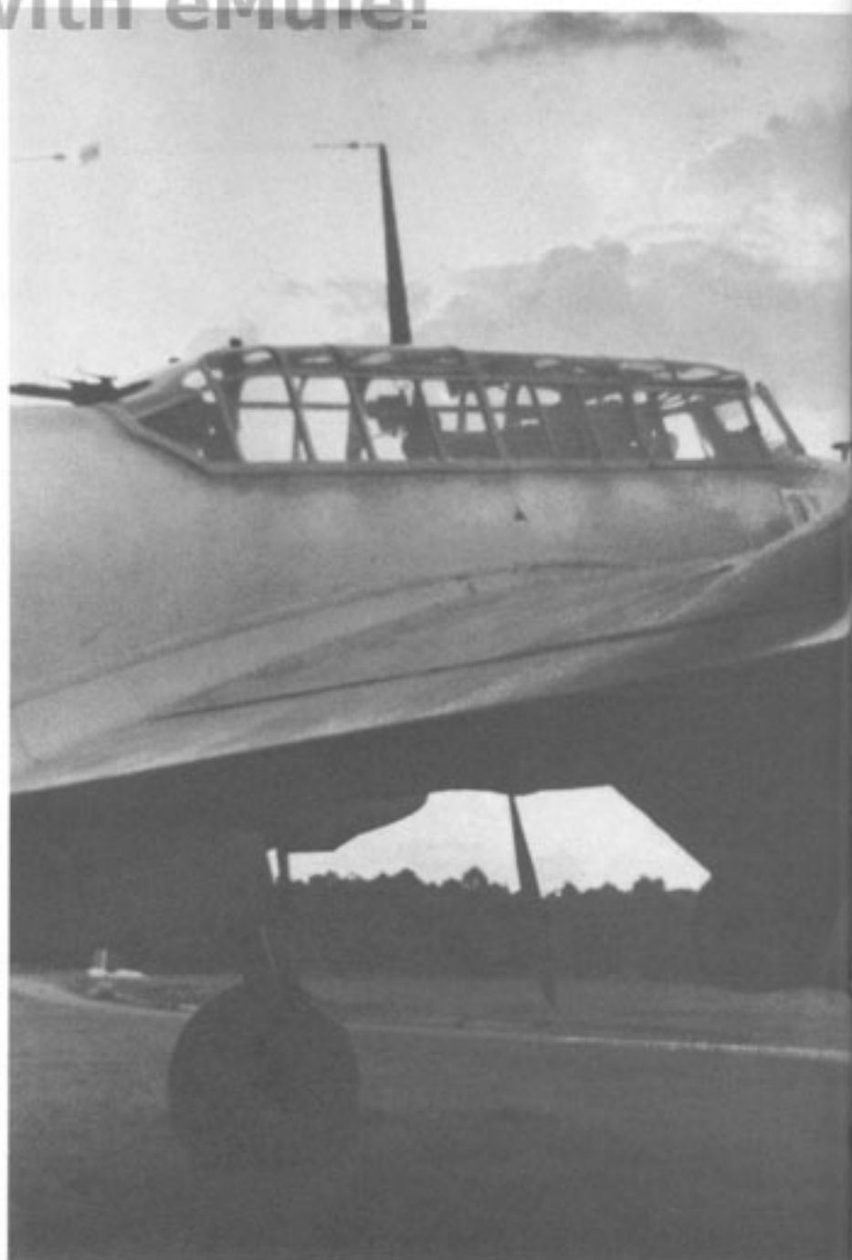
The almost vertical MK 108 cannon and the MG 81 Z free machine-gun made for a cramped rear cockpit in this Bf 110.
