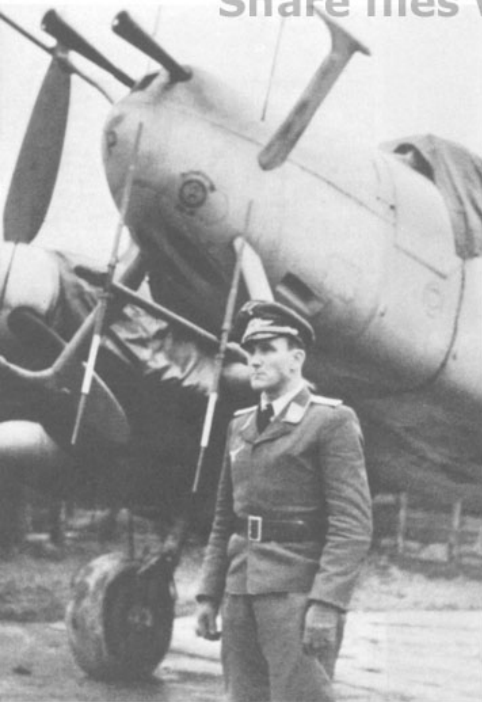
These muzzle flash dampers were one of many new modifications that gradually improved the nightfighters' effectiveness.
